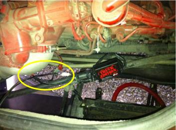
5) The switch can be routed inside the vehicle or once connected can be zip tied with the module and left in place.
