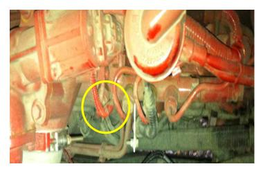
**3)** Follow the wiring out from the sensor until you reach a triangle-shaped connector. Unplug the 3-wire triangle-shaped connector.
