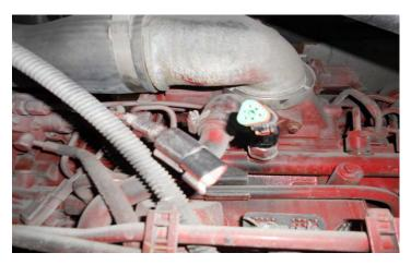
**4)** Connect the stock Cummins male connector to the female connector from the module. Connect the male Connector from the module to the stock Cummins female sensor.
