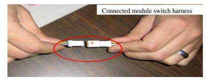
Remove the bypass plug from the Ag Diesel Solutions harness, and plug the harness into the module.
