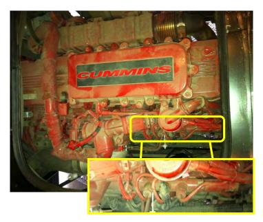
2) Locate the Fuel Pressure Sensor connected to the Fuel Rail.
